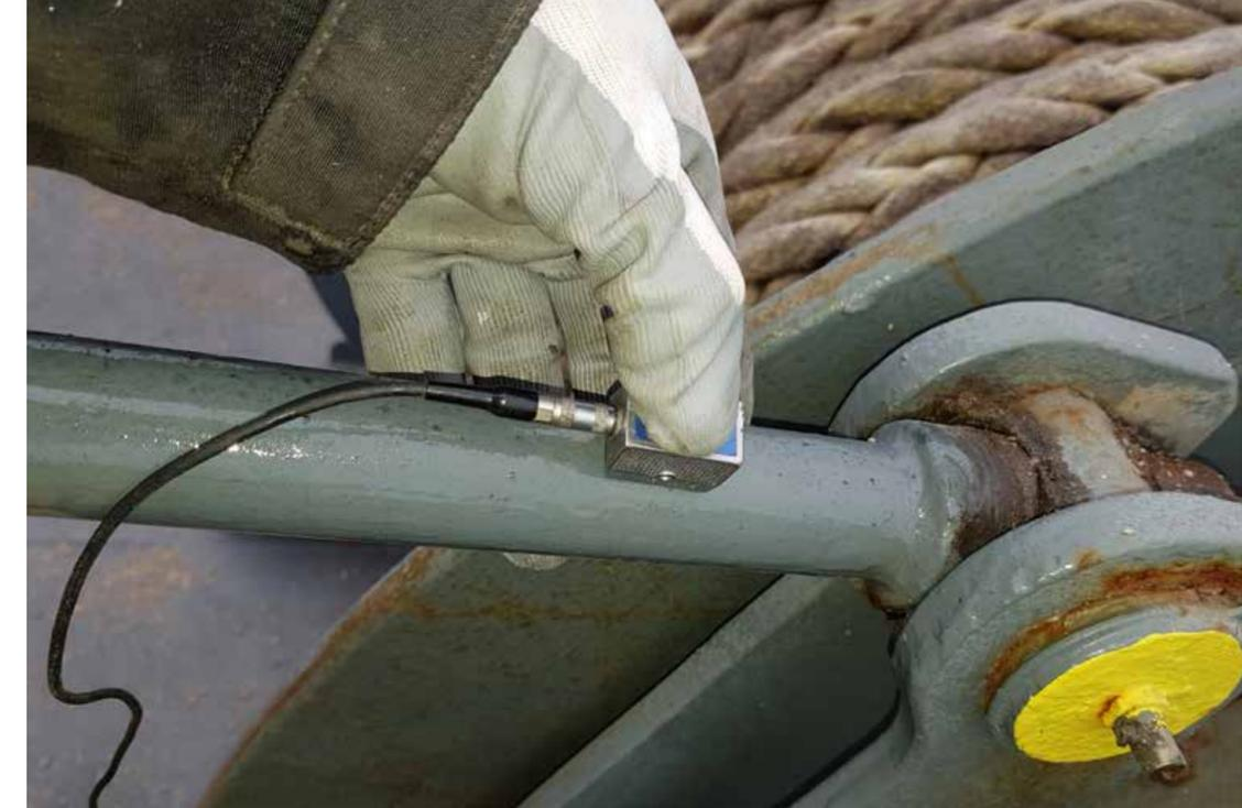
>> **Ultrasonic testing** This method will provide indications of surface and subsurface discontinuities, will determine by the use of the proper technique the depth and exact size of the damage in the material. Ultrasonic pulses are directed into the test object which produces echoes and reflections which then indicate the presence, absence and location of flaws, interface and/or discontinuities.
